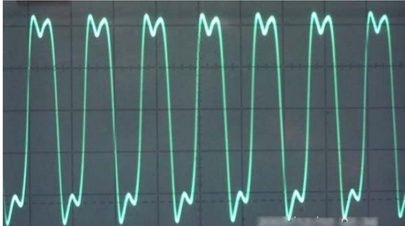
Kurvenform an Dummy , 40 m, 1 kW, o. Filter
